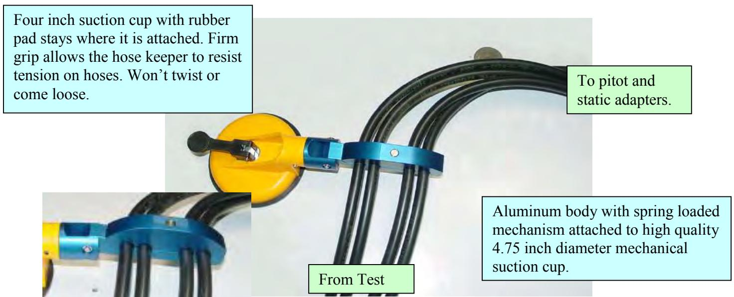
The hose grip assembly is also useful for hanging and organizing air lines and electric power cords at the edge of aircraft doors and emergency exit frames. Hose grip assemblies can reduce or eliminate the wear and damage to door seals that happens during airframe maintenance fabrication, and completion activities.
